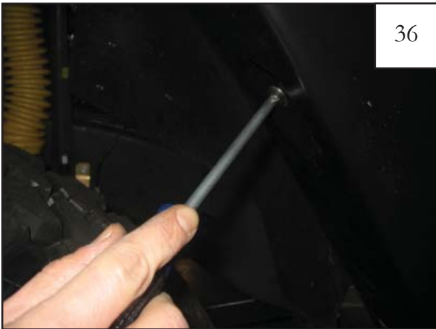
Install supplied Truss Head Screws through holes in wheel well and into #14 U-Clips installed in Step 26 (6 places). Ensure proper alignment of outer flare, inner flare and splash shield . Do not tighten at this time.
