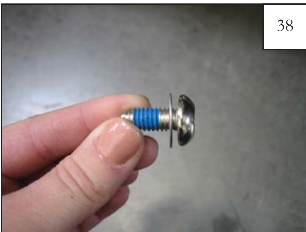
Slide a supplied .700" washer onto a supplied Torx Screw.
