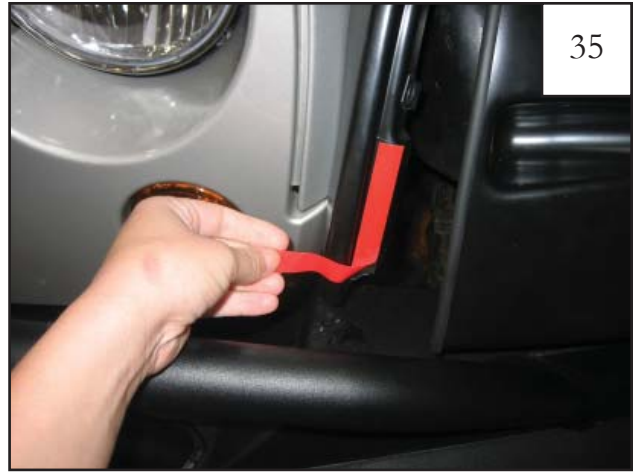
Fold tape liner tab attached to 1/2" peice of tape on outer edge of Inner Flare Piece upwards (do NOT peel liner from 1/2" tape in this step).
