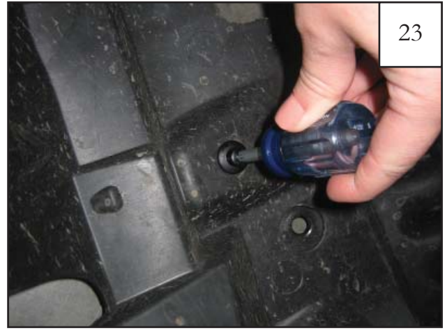
Using a Phillips screwdriver, reassemble inner structure and splash shield by installing supplied Plastic Phillips Head Tufloks (6 places). Use a pushing-twisting motion to install.
