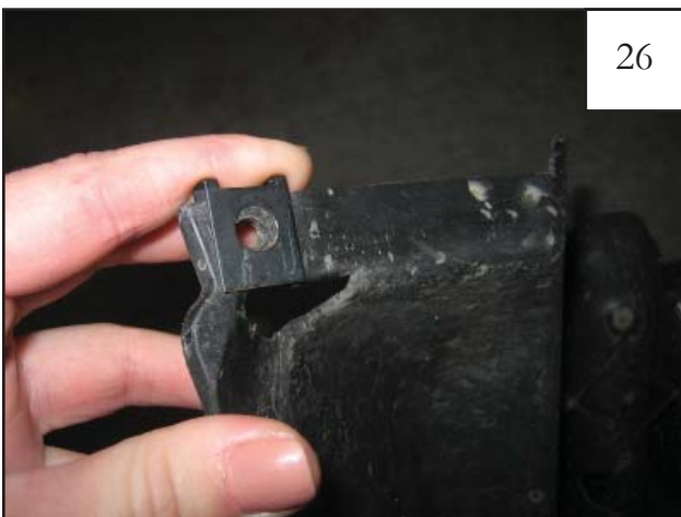
Install supplied #14 U-Clips over holes indicated in Step 27.
