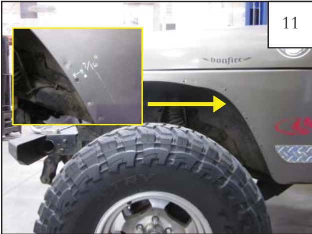
Locate the third factory hole from bottom of fender. Use a grease pencil to mark a hole for drilling 7/16" from center of factory hole, perpendicular with wheel well opening.
