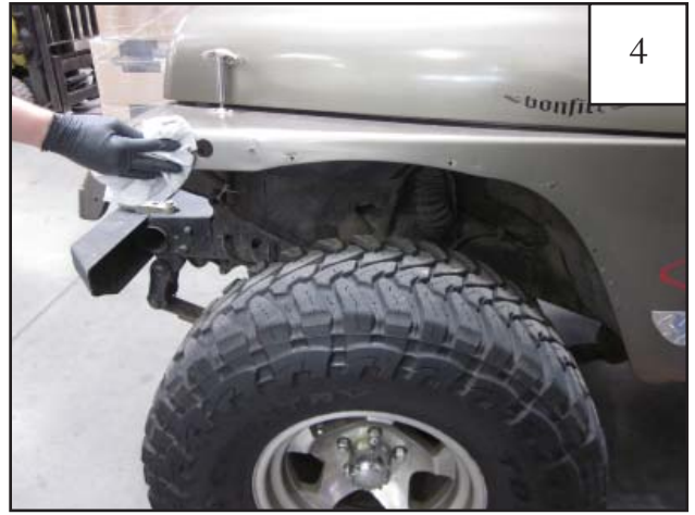
Remove the factory installed fender flares. Thoroughly clean the exposed metal fender with a damp cloth and dry.
