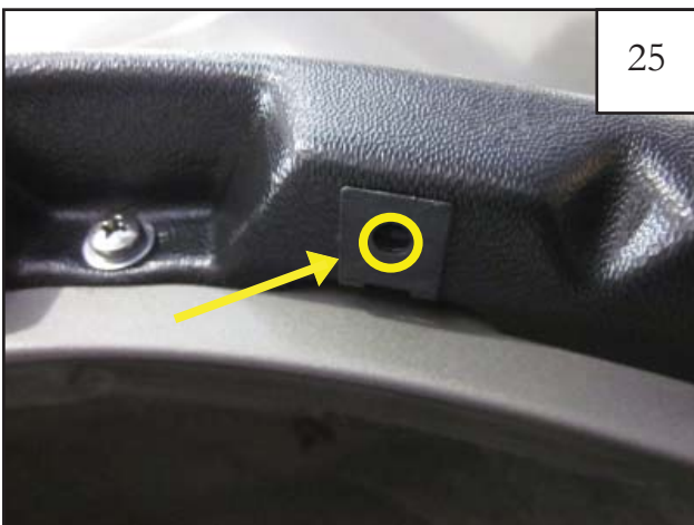
Before installing the outer flare, make sure that the Clips (CL1-0022) on the inner pieces are centered over the predrilled holes.
