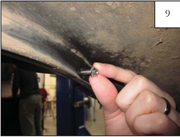
Step 2 Attach Nuts (NU1-0010) to the threads on the Screws (SW1-0053) and hand tighten.
