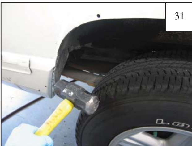
Use a small sledge hammer to flatten out sheet metal tabs. Remove the tire if desired to make hammering easier. Avoid bending or distorting outer sheet metal.
