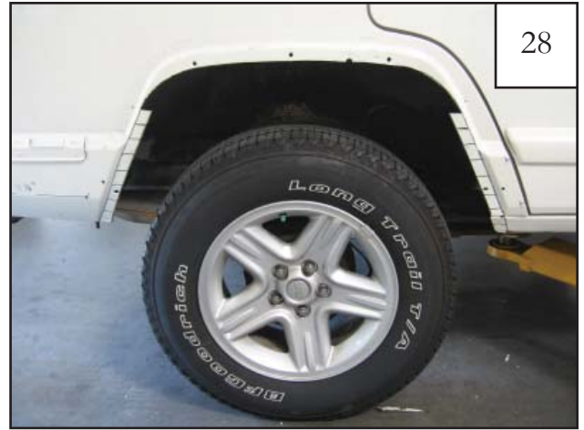
Fender should look like image shown after trimming and hammering.
