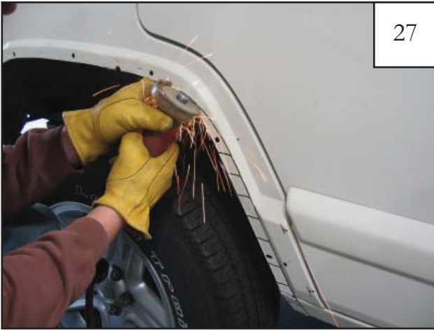
Use a cut off saw to cut the front fender along marked line. Do not cut any sheet metal past where the horizontal lines were marked in step 25.
