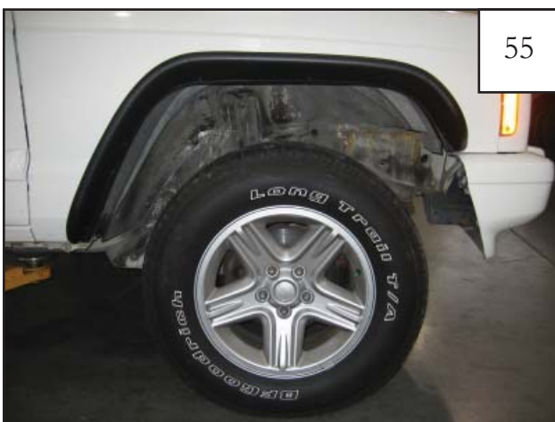
Completed front passenger's side flare installation.
