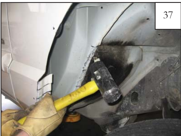
Use a small sledge hammer to flatten pinch weld against inner wheel well. Remove tire if needed. Use a ball peen hammer to further flatten and smooth out pinch weld.
