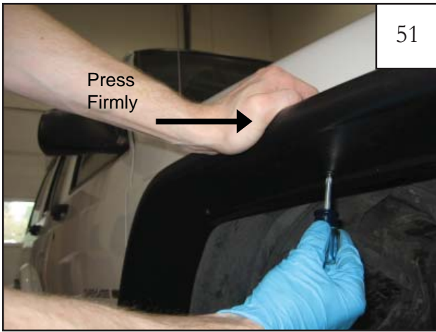
Tighten the #8 pan head screws by firmly pressing the flare toward the vehicle while tightening.
