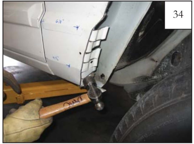
Use a hammer to flatten out sheet metal tabs. Avoid bending or distorting outer sheet metal.
