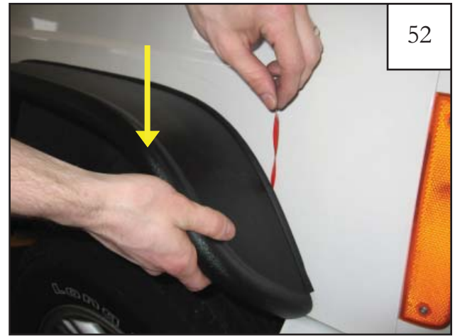
Peel outer tape liner from the double-tape edge trim. Push down lightly on the fender flare to create a small gap between the sheet metal and the edge trim. This makes it easier to pull the red liner.
