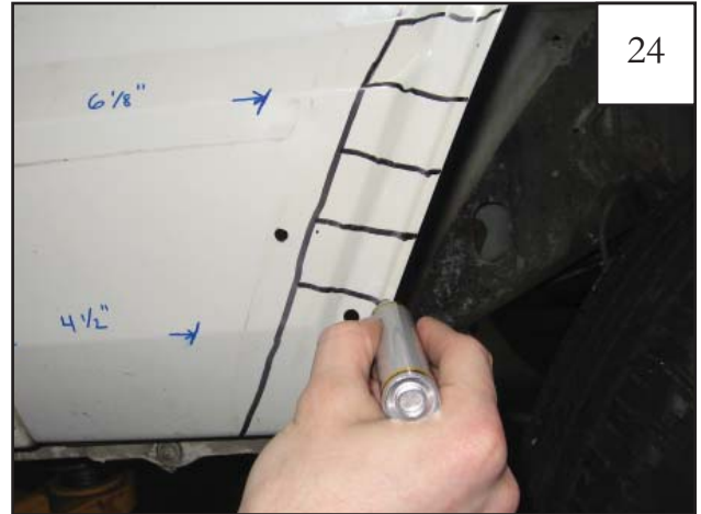
24 Remove inner pieces. Mark horizontal lines 1.5" apart starting on lower rear style line of sheet metal and ending on upper horizontal style line in sheet metal.
