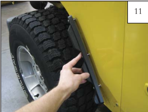
Secure inner pieces D2 (and P2 for passenger side installation) to the sheet metal using the following 2 Steps: Step 1 Line up the M5-.8 machine screws with the factory hole locations.
