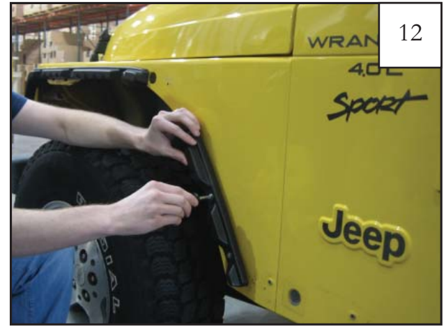
Step 2 While holding the inner piece in place, use a #2 Phillips bit to tighten the M5-.8 machine screws into the factory mounted nuts.
