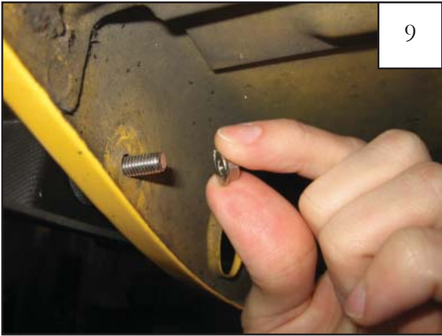
Step 2 Attach flange nuts to the threads on the M5-.8 machine screws and hand tighten.
