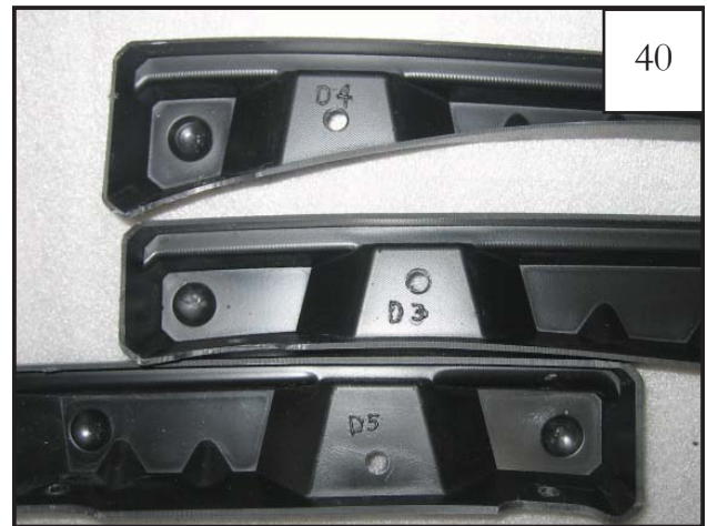
Locate the new flat flare rear inner pieces. The driver side rear inner pieces are marked D3, D4, and D5. The passenger side rear inner pieces are marked P3, P4, and P5.
