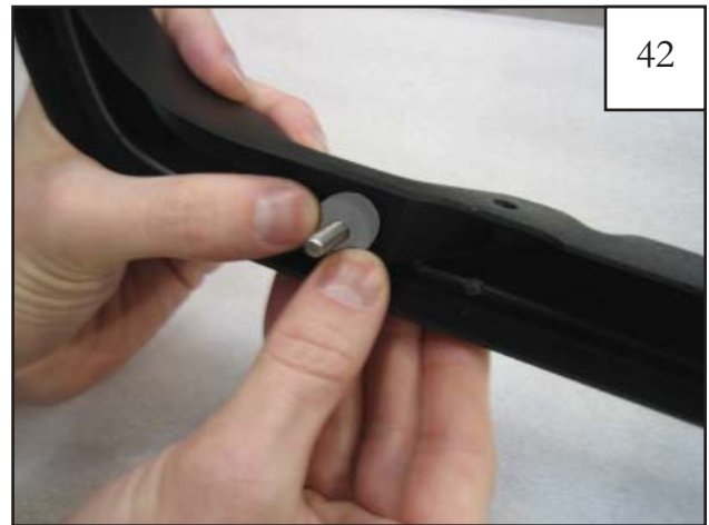
Push the rubber spacer and M5-8 machine screw together until they are both tight against the inner piece. Spacer has been lightened in picture for visibility.
