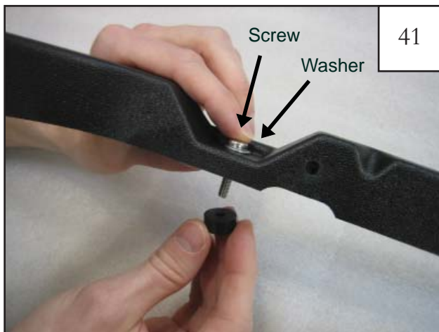
Put an M5-8 machine screw and washer through the top holes of the inner pieces and secure with a 1/4" rubber spacer on the underside of the inner piece.
