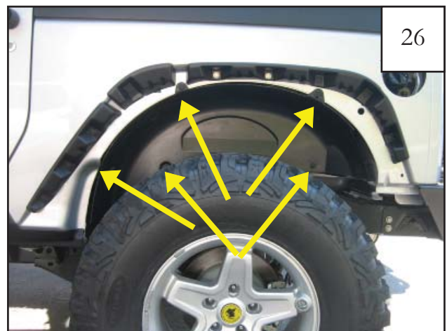
Reinstall modified splash shield using supplied 1/4" Panel Retainers (5 locations).
