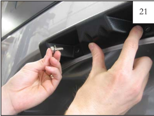
Step 3 Slide a .700" Washer onto 5/16" Hex Head Bolt. Insert a bolt/washer assembly through inner flare piece and fender in frontward two locations and secure with 5/16" Nylok Nut. Start the bolts but do not tighten.
