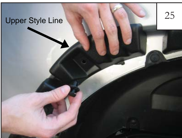
Step 2 While holding the inner piece in place, install a plastic push retainer. Inner piece should rest along upper style line of sheet metal radius and not below it: see step 18.
