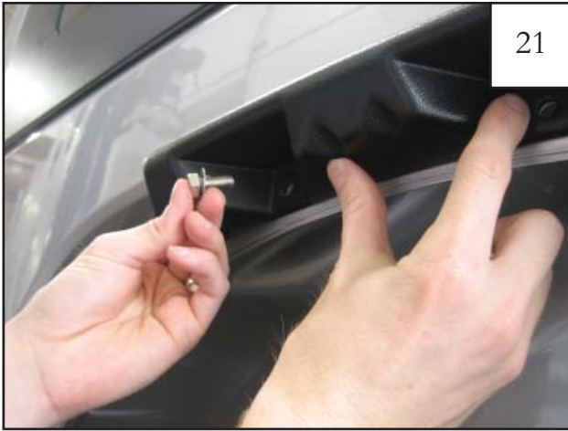
Step 3 Slide a .700" Washer onto 5/16" Hex Head Bolt. Insert a bolt/washer assembly through inner flare piece and fender in frontward two locations and secure with 5/16" Nylok Nut. Start the bolts but do not tighten.
