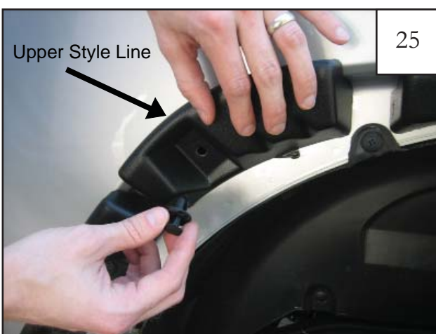
Step 2 While holding the inner piece in place, install a plastic push retainer. Inner piece should rest along upper style line of sheet metal radius and not below it: see step 18.
