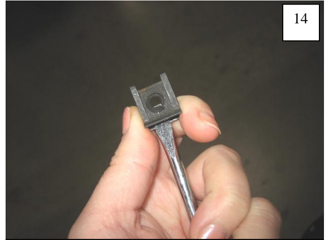
Use a flat head screwdriver to spread supplied #14 U-Clips for ease of installation.
