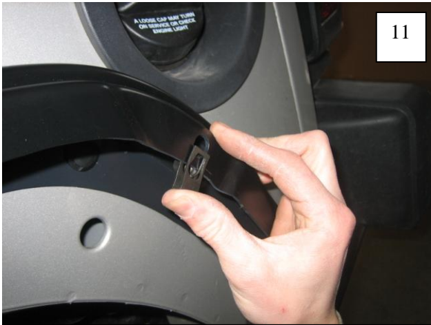
Install supplied Threaded Clips, with the thread side in, over holes in Inner Flare Piece (8 places).
