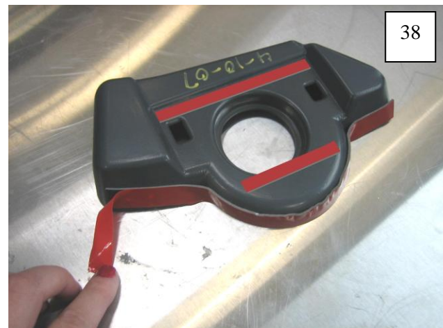
Peel liner completely from two pieces of 1/4" tape located on face of Light Pocket Inner Piece. Fold tape liner tab attached to long 1/2" piece of tape upwards (do NOT peel liner from 1/2" tape in this step).
