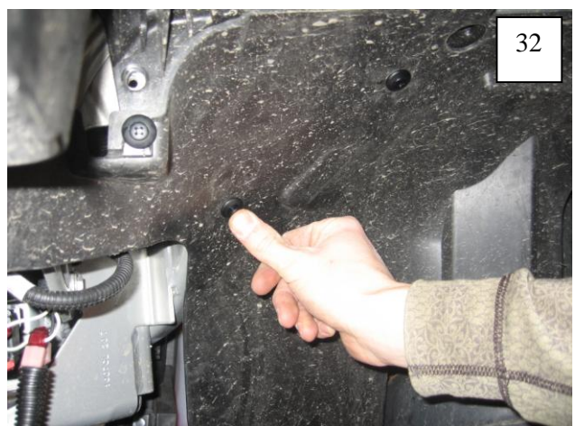
Install a supplied Plastic Phillips Head Tuf-Lok in hole located toward the front of the splash shield.
