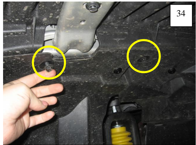
Reinstall two factory bolts as shown.
