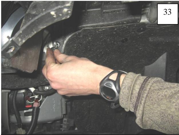
Reinstall the factory bolt at front of splash shield.
