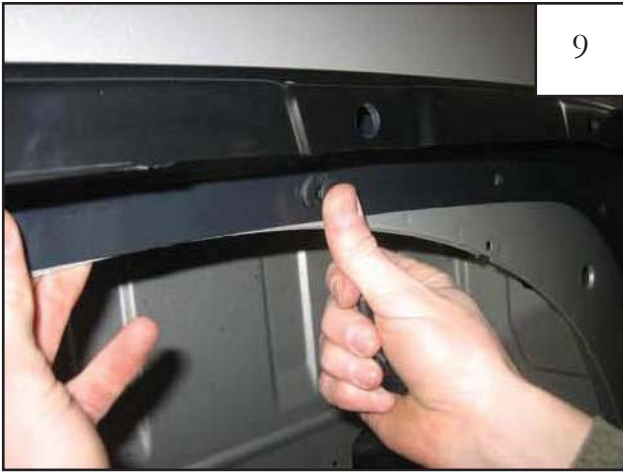
Position Inner Flare Piece on fender, aligning existing 5/16" holes in Inner Flare Piece with holes in fender. Install supplied Plastic Push Retainers (RV1-P006) (9 places).
