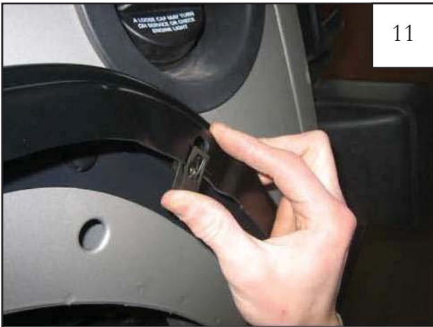
Install supplied Threaded Clips (NU1-0017), with the thread side in, over holes in Inner Flare Piece (8 places).
