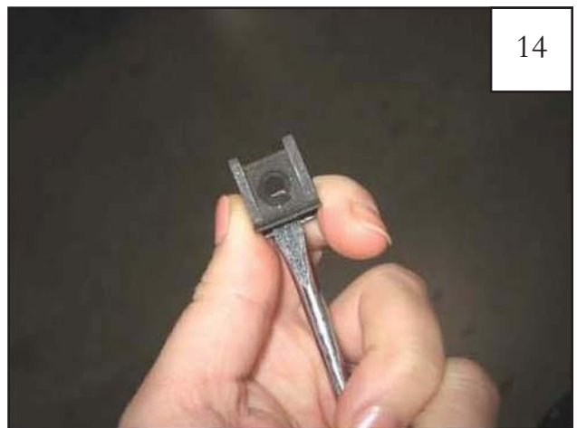
Use a flat head screwdriver to spread supplied #14 U-Clips (NU1-0013) for ease of installation.
