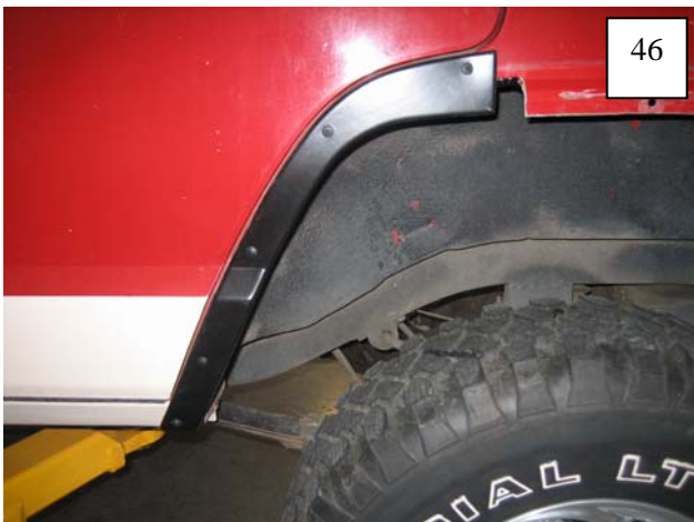
Open door. Install cover piece over "dog leg" using five supplied drill screws. Place drill screw in indent in part and drill into sheet metal. NOTE: Some trimming may be required.
