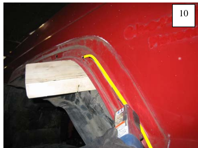
Starting at bottom rear of fender, cut along lines using a reciprocating saw or grinder. Note: it is helpful to use a block of wood to separate the fender from the splash guard, which will be trimmed later.
