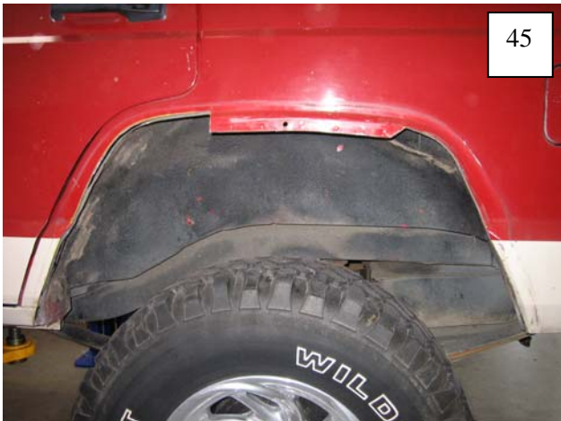
The fender should look like this. Some additional grinding may be needed. Optional: use caulking to seal all cut edges and seams.
