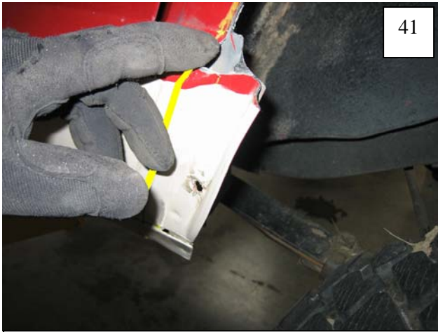
Along front fender well edge, cut through sheet metal down to the flare-out feature at the bottom.
