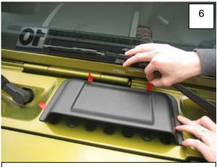
Maintaining part placement, begin pulling tape tabs while applying downward pressure to part.
