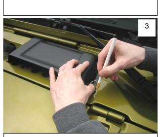
Once positioned, use a grease pencil to lightly trace around edges of part.
