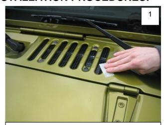
Use supplied alcohol wipe to wipe the installation area.
