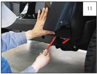
From rear to front, pull tape liner tab 6. Press firmly on the part following tape liner removal. *NOTE:* Refer to step 1 for additional tape tab identification.
