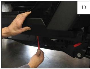
From rear to front, pull tape liner tab 5. Press firmly on the part following tape liner removal. *NOTE:* Refer to step 1 for additional tape tab identification.
