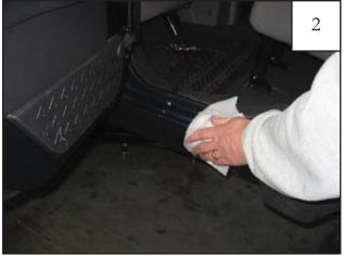
Open vehicle door. Clean all dirt and debris from vehicle door sills, rocker panel, and beneath flares if installed. Then use supplied alcohol wipe where part will be. NOTE: Temperature should be at least 60°F for proper tape adhesion.
