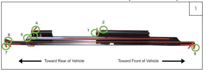
Using a marker, number the tape tabs for the tape liners as shown:
