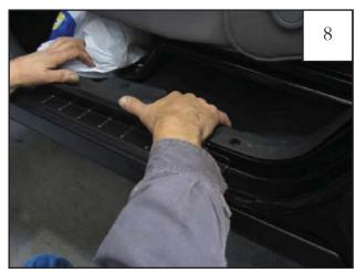
Press down firmly on part along the length of the sill.
