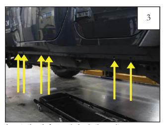
Locate the six factory holes in the rocker.
