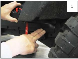
Place part on vehicle, making sure to line up edges of part with edges of vehicle and hole in part with clips installed in step 4. Ensure that all tape tabs are accessible.
