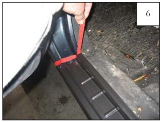
At the front door sill, pull 1/2" tape liner tab 1. NOTE: Take care not to catch tape liner of other pieces of tape and accidentally pull their liners off as well. NOTE: Refer to step 1 for additional tape tab identification.
