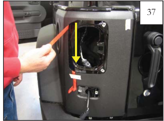
Pull tape liner 10 downward. NOTE: Refer to step 24 for tape liner tab numbering.
