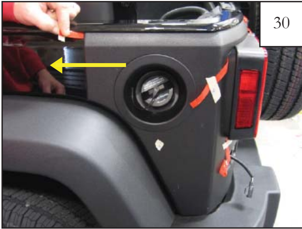
Pull tape liner 5 left toward the front of the vehicle. Press side of part firmly for proper tape adhesion. NOTE: Refer to step 24 for tape liner tab numbering.
