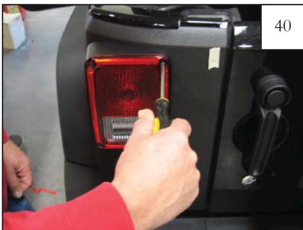
Using a #2 Phillips screwdriver, reinstall tail light.
