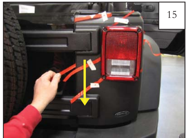
Pull tape liner 2 downward. NOTE: Refer to steps 8 & 9 for tape liner tab numbering. Using a #2 Phillips screwdriver, remove the light again.
