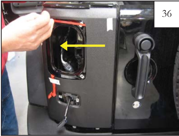
Pull tape liner 9 for the 1/4" tape to the left toward the driver side of the vehicle. NOTE: Refer to step 24 for tape liner tab numbering.
