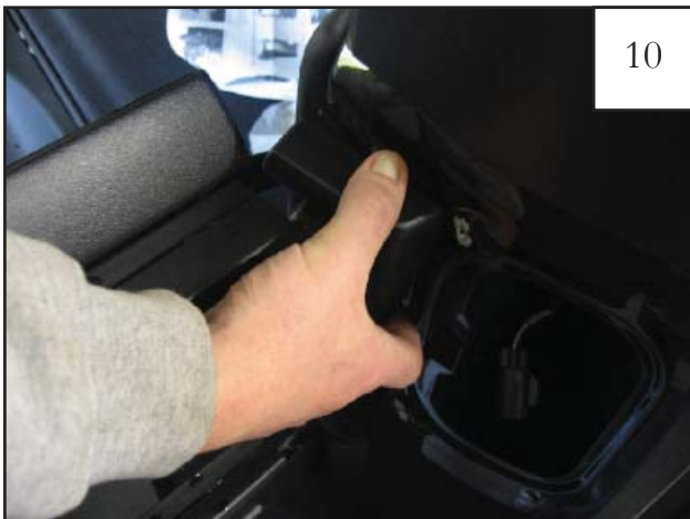
Slide covers off door hinges.
