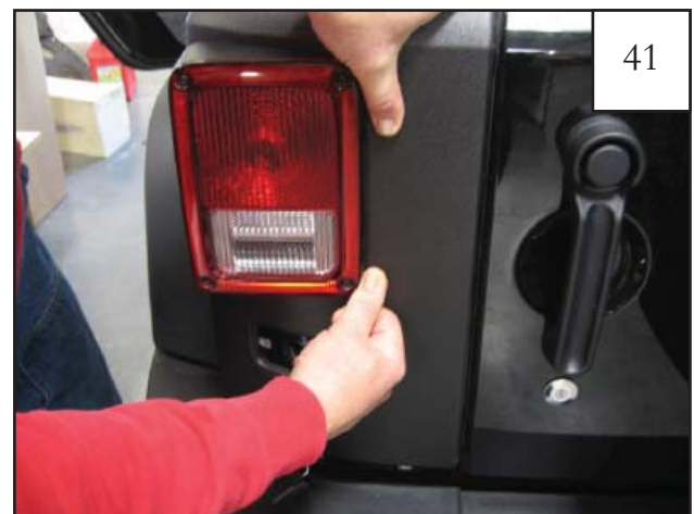
Once all tape liners are peeled, press down on entire again applying 30 PSI to the taped areas. Take special care in pressing down around the tail light. NOTE: The tape reaches maximum adhesive bond after 24 hours of contact. Do not wash vehicle for 24 hours.
