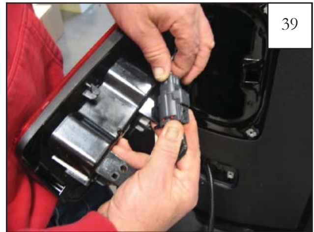
Reconnect light connector of tail light.
