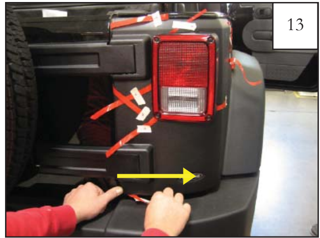
Pull tape liner 1 to the right toward the passenger side of the vehicle. NOTE: Refer to steps 8 & 9 for tape liner tab numbering.
