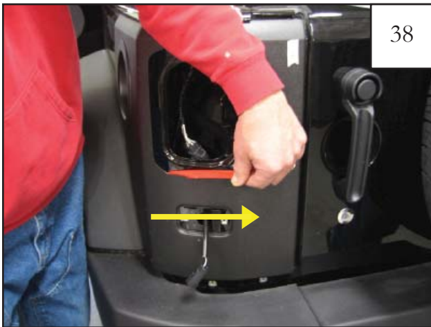
Pull tape liner 11 to the right toward the passenger side of the vehicle. NOTE: Refer to step 24 for tape liner tab numbering.
