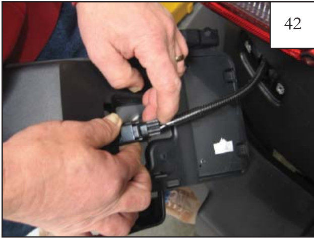
Reconnect light of license plate frame.
