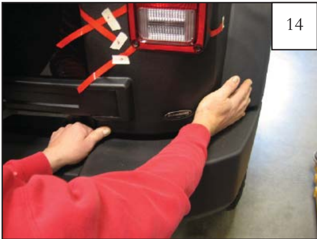
Press down firmly around the entire lower line of the part where the tape was removed.
