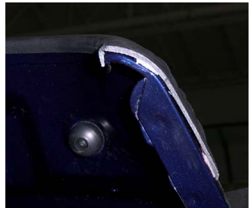
Photo #2 – Hood Protector lip over edge of hood
