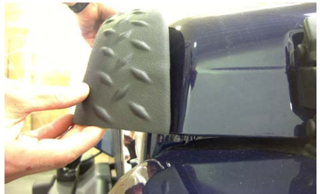
Photo #1 – Hood Protector placement
