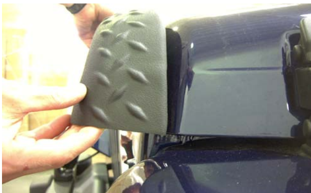
Photo #5 – Hood Protector placement
