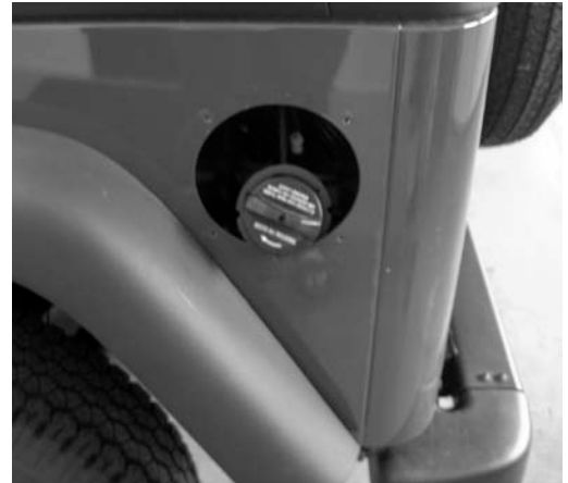
Figure #1 – Remove Gas Tank Outer Flange
