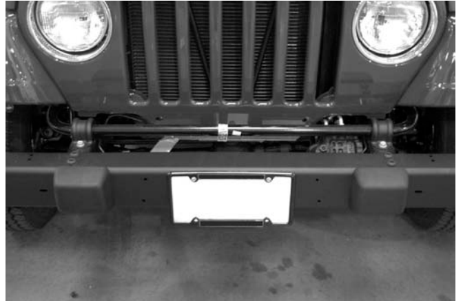
Figure #8 – Factory Front Panel Removed
