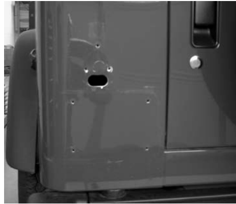
Figure #2 – Remove Tail Light & License Plate
