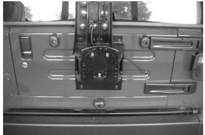
Figure #3 – Remove Spare Tire
