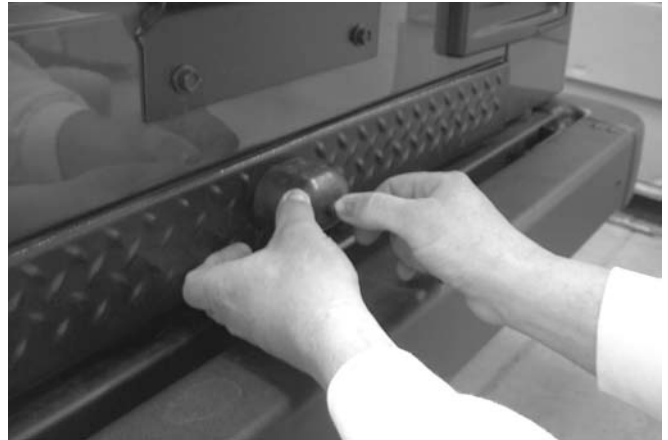
Figure #5 – Reinstall Tire Stop & Tire
