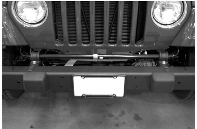
Figure #8 – Factory Front Panel Removed
