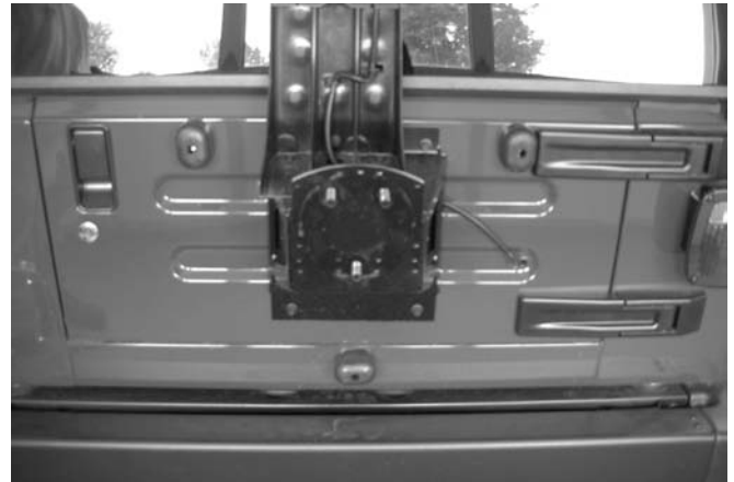
Figure #3 – Remove Spare Tire
