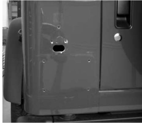
Figure #2 – Remove Tail Light & License Plate
