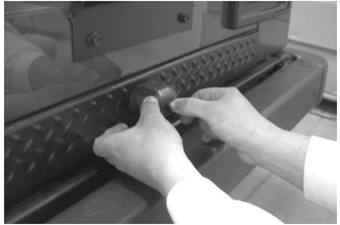
Figure #5 – Reinstall Tire Stop & Tire
