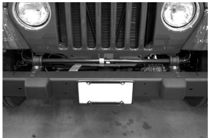
Figure #8 – Factory Front Panel Removed
