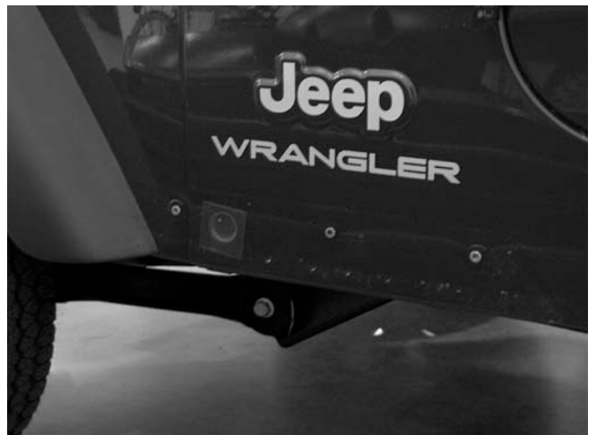
Figure #6 – Remove Stone Guard
