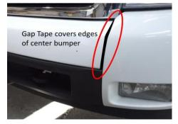
3. Being careful not to let the tape touch down on the bumper surface, start from either the left or right side of the bumper by tucking the leading edge under the grill and butting the edge trim against the OEM corner plastic bumper. Continue across the bumper to the other side, lightly tucking the top of the cover under the grill area.
