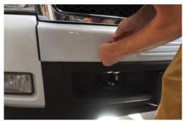
6. When satisfied with the position of the BumperShell, begin putting firm pressure on the taped areas of the cover. Start with the vertical surface, leaving the tape on the top surface for last. This will allow for easier installation of the BumperShell.
