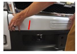
5. Ensure that the bumper cover is properly positioned. (There should be no, or very little bumper surface visible at this point). Re-adjust, as necessary.
