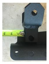
Step 2: Hold the bracket tight against the weld and use the 5/8" drill bit to make a center point indentation in the gusset. (Using the 5/8" bit will ensure the indentation is the center in the hole). As seen below
