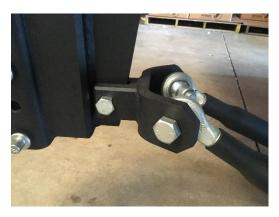
Step 6: Mount the stabilizer bars to the bracket on the hitch. This will allow you to gauge the location of the frame brackets.
