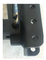
Step 3: Once you have an indentation use the  $\frac{1}{2}$  drill bit to make the first hole all the way through the gusset. As seen below (Be sure to drill the hole as straight as possible)
