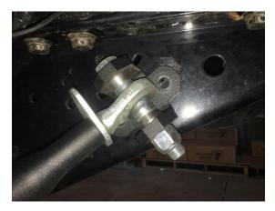
Step 9: When you have located where you will need the holes use the  $\frac{1}{2}$ " bit to drill the holes in the frame.
