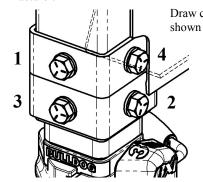
**Outer Tube** Draw coupler into position according to the pattern shown and then torque pinch bolts to 200 ft-lbs. Gussets - Top & Bottom **Pinch Bolts** Max. Extension = 2.6" from Fully Retracted Position BULLDOG must face tow vehicle
