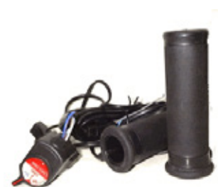
INCLUDES HI-LOW-OFF TOGGLE SWITCH. SAME AS 5-183-1, ONLY SMOOTH 14.2V, 0.79A, 11WATT
