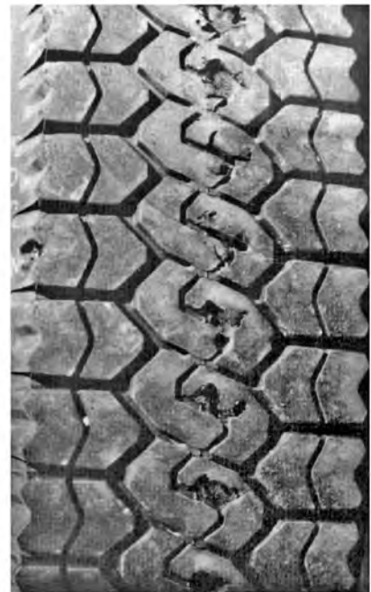
Example of Dyno Damage
