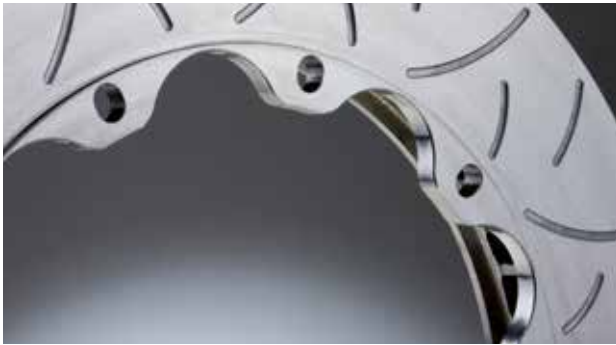
OH - Standard fixing with oval holes
