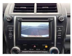
**Step 8: Reverse Feed (If Req'd)**. In Scion and Tacoma vehicles you may need to supply the reverse signal to the radio. Use the loose green wire supplied in this kit. First insert the terminal end into pin-2 of the white 24-pin radio connector. See page two of these instructions for your vehicle reverse wiring location.
