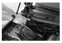
Disconnect the wiring connectors by pressing/squeezing down on the red release buttons on the top of the connector. Remove all the connectors from the ECU. (see photo 5)
