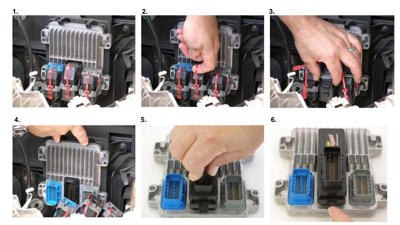
Step 5: Reinstall the computer on the firewall and reattach the connectors to the computer. Be sure to lock the connectors in place with the gray connector handles and the red securing straps. Reconnect the battery cable, then start the vehicle and make sure the check engine light is not on and the vehicle is running normally. This completes installation. Please keep these instructions for future reference.
