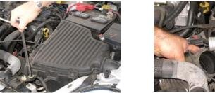
Step 3: There are four connectors located on the front of the computer. Disconnect all four connectors from the computer by pressing down on the release buttons on each wiring harness plug. Next remove the three bolts holding the computer to the vehicles body.
