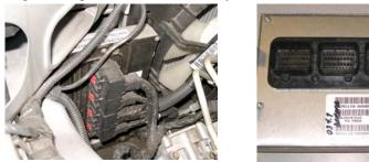
Step 4: Lay your computer on a flat surface and plug your Jet Module into the connector shown in the pictures above and below. Be sure the module fully seats or the vehicle may not start. Now with the module installed in your computer, mount the computer back in the vehicle and plug all the wiring harness plugs back into you computer and the Jet Module.
