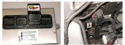
Step 5: Reconnect the negative side terminal of the battery. Start your vehicle and make sure the "service engine soon" light is not on and the vehicle is running normally.
