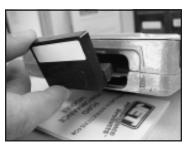
**Step 2**Plug Jet Module onto connector.
