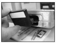
**Step 2**Plug Jet Module onto connector.
