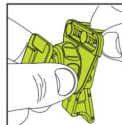
Remove the body of the vent clip by sliding the spring vent clip to the center of the body and pulling it through.
