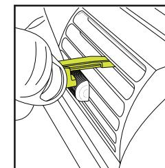
Pull back on the spring slide clip compressing it completely.
