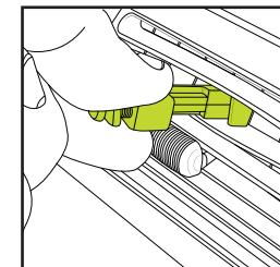
Push the entire clip in slightly so the hook clears the louver. Twist the clip 90 degrees and pull away from vent to remove.
