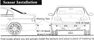
First locate where you are goingto install the sensors and place a piece of masking tape Measure and mark the positions of the holes
