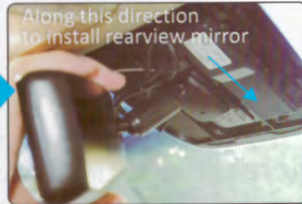
Along this direction to install rearview mirror
