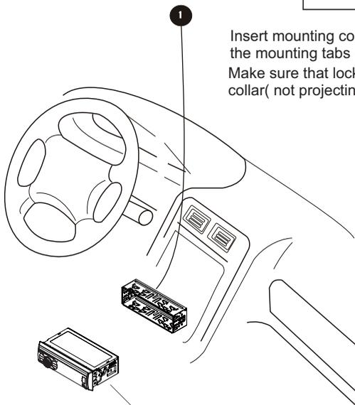
1 Insert mounting collar into the dashboard and bend the mounting tabs out with a screwdriver.
