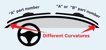
Bosch ICON™ blades use exclusive tension spring arcing technology to create a fit that is custom-contoured to the curvature of each side of the windshield. The correct blade for a particular vehicle is based on a combination of the blade length and the curvature of the windshield.
