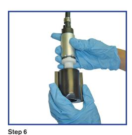
Compare new pump inlet size to original pump. If necessary, attach filter screen adapter to the new pump. Then fit fuel pump into rubber support.
