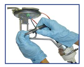
Attach fuel pump to fuel inlet tube with supplied clamps. Tighten clamps. Remember: Do not reuse fuel pulsator.
