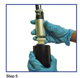
Connecthose,clampsandsuppliedwiring harness to the pump.
