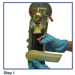
Note and nark the position of existing fiter strainer. Remove the existing filter screen.
