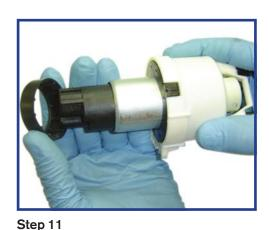
Assemble rubber ring support over the pump.
