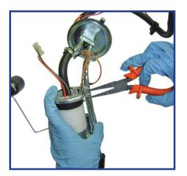
Reassemble the attachment support to the new pump and onto the module.
