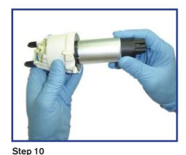
Mount new fuel pump into housing.
