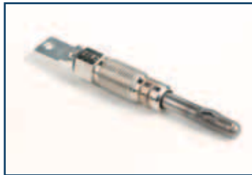
Glow Plugs damaged due to over voltage
