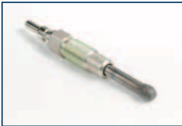
Glow Plugs damaged due to over voltage
