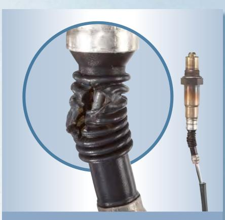
**State of oxygen sensor:** The molded cable tubing is damaged.
