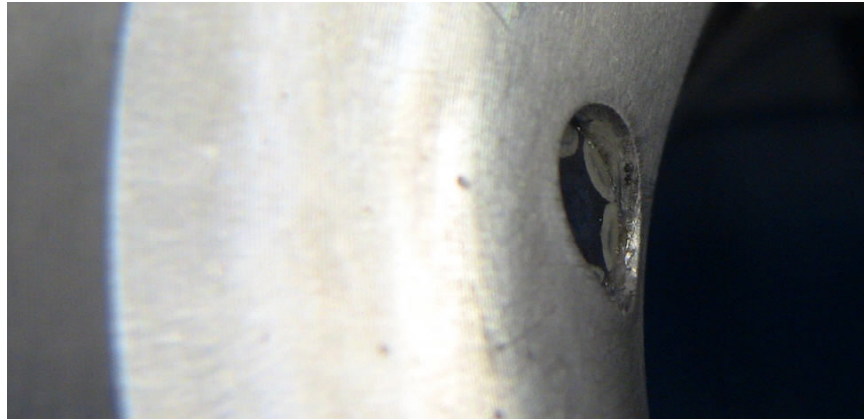
Figure 69: Example of Sensor Tip that is Not Sufficiently Deep
