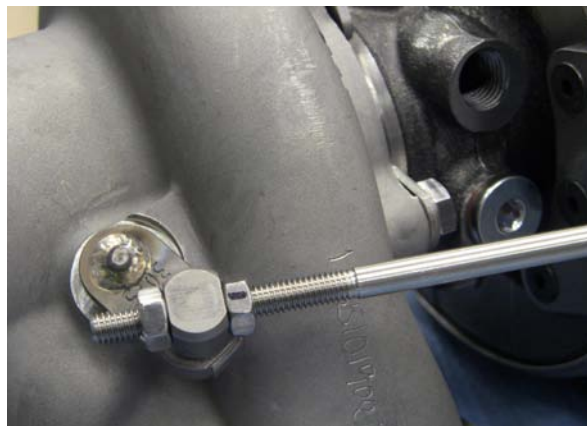
Figure 84: Line Drawn On Nut to More Easily Count Turns (2mm Preload Added)
