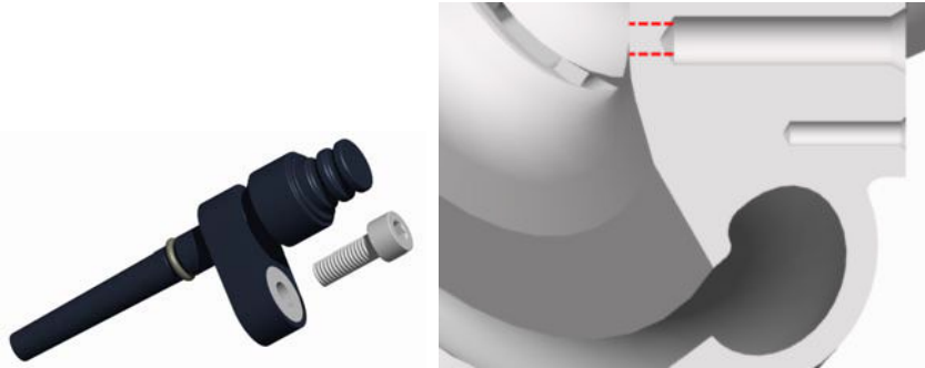
Figure 65: Speed Sensor Kit (Left) and Hole Drilling Schematic (Right)
