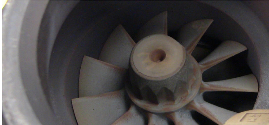
Figure 39: Gamma-Ti Wheel at End of Successful Thermal Durability Test
