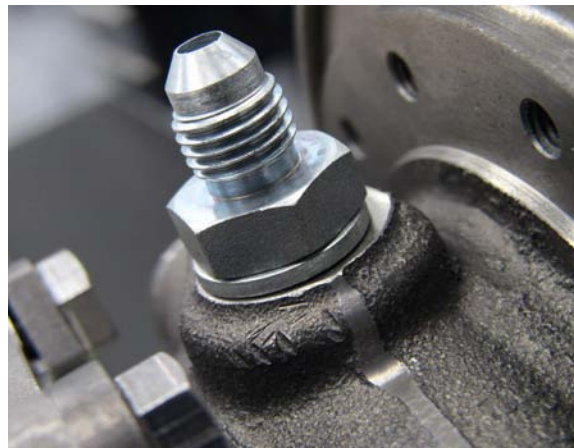
Figure 30: -4AN Oil Inlet Fitting (Supplied)
