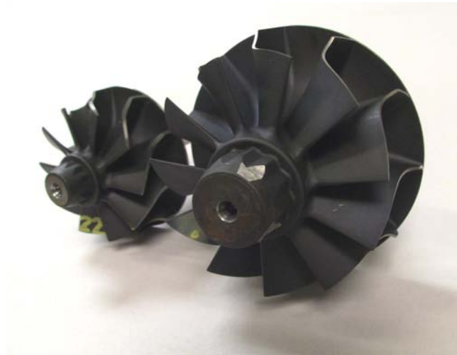
Figure 36: Gamma-Ti Turbine Wheels (55mm and 74mm Examples)
