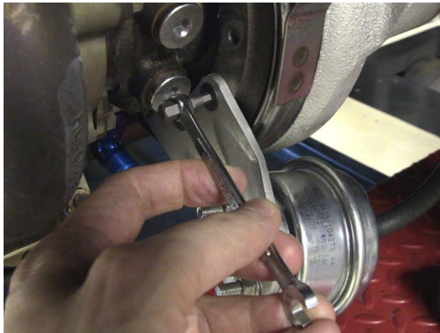
Figure 74: An Alternative to the Typical Angled Hex Wrench (in this example, only 2 of the 3 bolts are being used due to hanging the bracket off the mounting pad)
