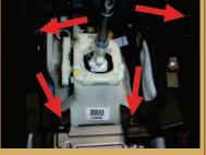
Remove the screw holding the center console.
