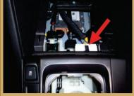
Remove the screw holding the trim under the steering column.
