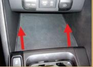
Remove the screws securing the center console.
