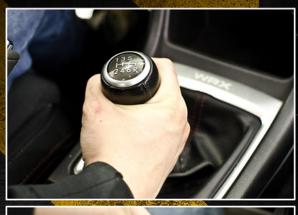
REMOVE OEM SHIFT KNOB BY UNSCREWING IT COUNTER-CLOCKWISE.
