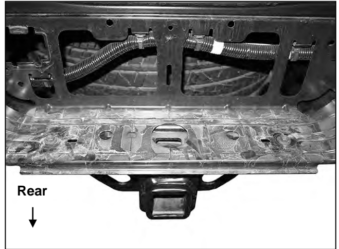
(Fig 4) Models with receiver hitch, remove plastic cover from top of bumper
