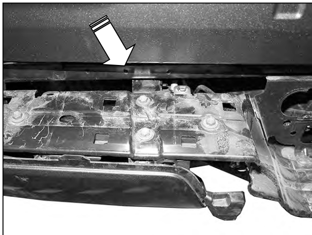
(Fig 5) Models with receiver hitch, remove the hex bolts attaching bumper to top of hitch
