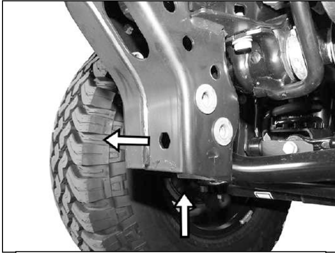
(Fig 4) Models with open hex-shaped hole in frame-insert 10mm Bolt Plate up into open end of frame and out through hex hole in front of frame (passenger/right side of frame pictured)
