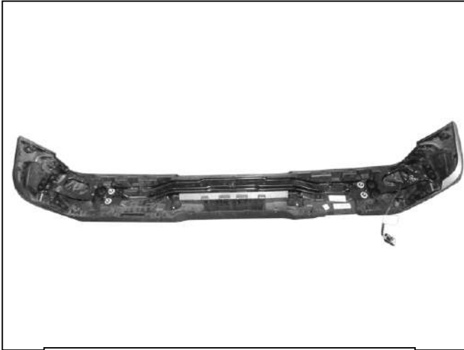
(Fig 10) Disassemble factory bumper to remove sensors and wiring harness
