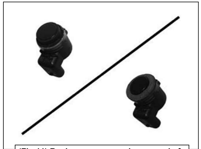
(Fig 11) Replace sensor washer on end of sensor with provided larger Foam Washer
