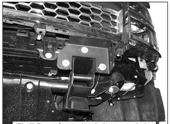
(Fig 7) Reuse factory hex bolts to attach the driver/left Frame Bracket to frame mount
