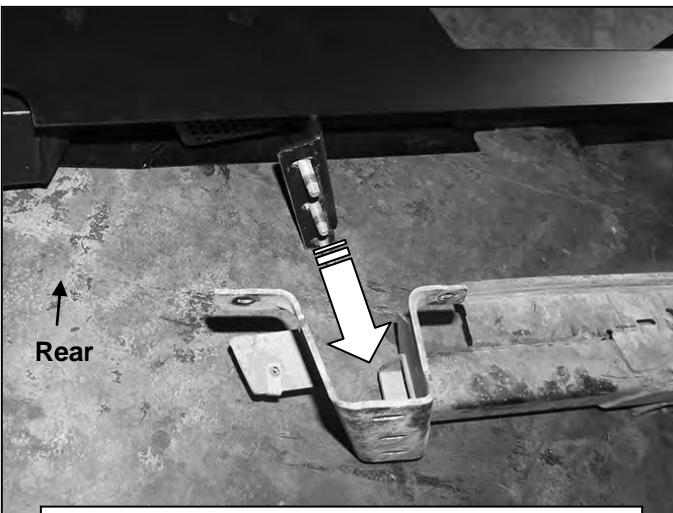
(Fig 5) On models with factory receiver hitch, slide Bumper up against the hitch. Insert triple bolt plates through bumper and hitch
