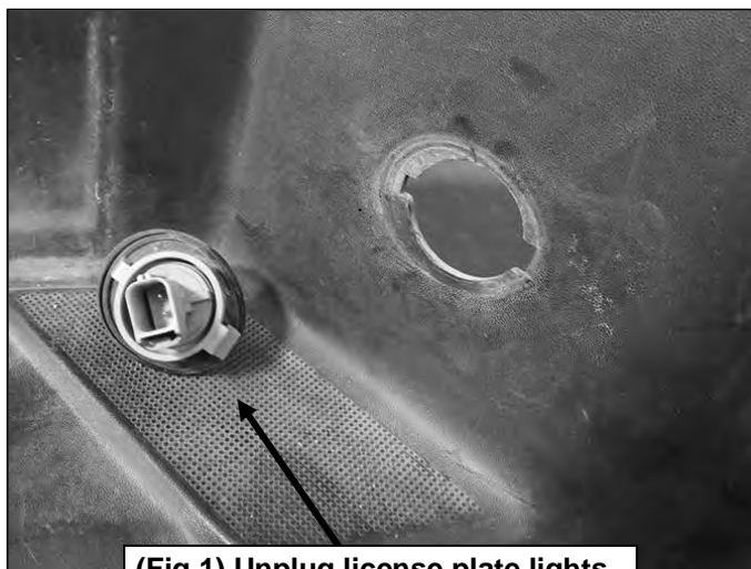
(Fig 1) Unplug license plate lights
