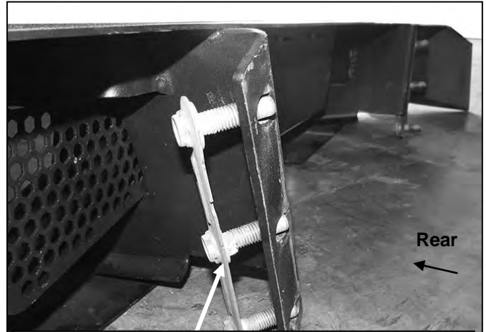
(Fig 4) On models without received hitch, reuse triple bolt plate to attach bumper to ends of frame
